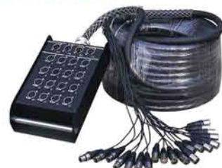
• AP-SC2448 > 20 channel stage box > Box end: 16xlr female+4xlr male > Span end:16xlr male+4xlr female > Balanced cable available with different length
